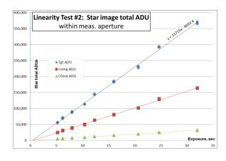
Figure 5: Linearity test (integrated ADU vs exposure duration).
