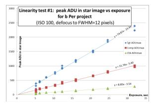
Figure 4: Linearity test (peak ADU vs. exposure duration).
